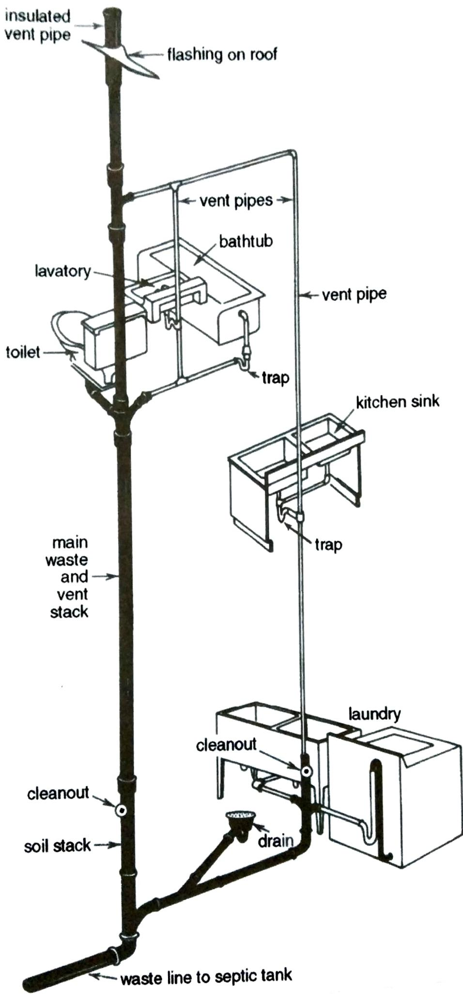
Figure 1. House plumbing includes waste and vent pipes, as well as well plumbing fixtures.
